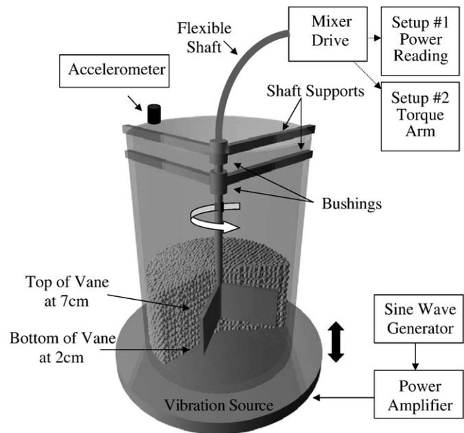
Fig. 1. Schematic of the experimental apparatus.
