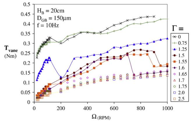
**Fig. 5.** Vane probe torque,  $T_{\text{vane}}$ , for increasing vane speed,  $\Omega$ .  $T_{\text{vane}}$  for  $\Omega > 200$  rpm is calculated from  $P_{\text{vane}}$  and demonstrates the similar behavior to  $P_{\text{vane}}$ . Note that torque is not constant for each  $\Gamma$ .  $T_{\text{vane}}$  dependence on  $\Omega$  indicates that the vane contributes to the state of the bed.
