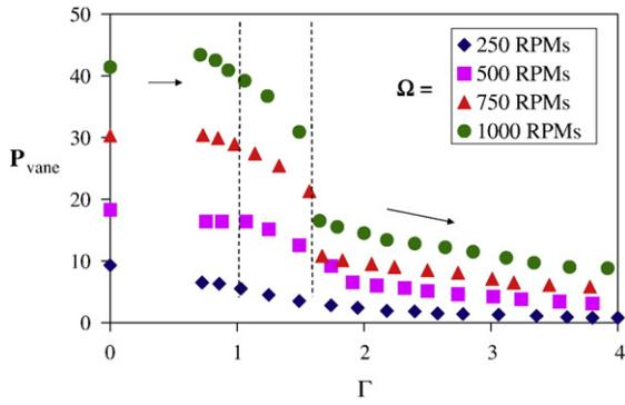
**Fig. 7.** Vane probe power draw,  $P_{\text{vane}}$ , for increasing dimensionless vibration acceleration,  $\Gamma$ . The granular bed state behavior shown by  $P_{\text{vane}}$  for  $\Gamma$  increase is similar to  $\Omega$  increase in Fig. 2.
