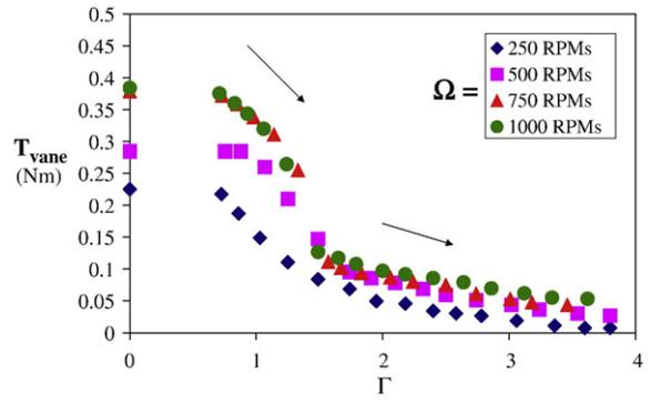
**Fig. 9.** Vane probe torque,  $T_{\text{vane}}$ , for increasing dimensionless vibration acceleration,  $\Gamma$ . The granular bed state behavior shown by  $T_{\text{vane}}$  for  $\Gamma$  increase is similar to  $\Omega$  increase in Fig. 5.
