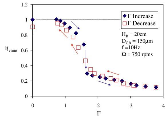
**Fig. 10.** Dimensionless vane power,  $\eta_{\text{vane}}$ , for increasing and decreasing dimensionless vibration acceleration,  $\Gamma$ , at  $\Omega = 750$  rpm. Hysteresis occurs for increasing vs. decreasing the dimensionless vibration acceleration at constant vane speed.
