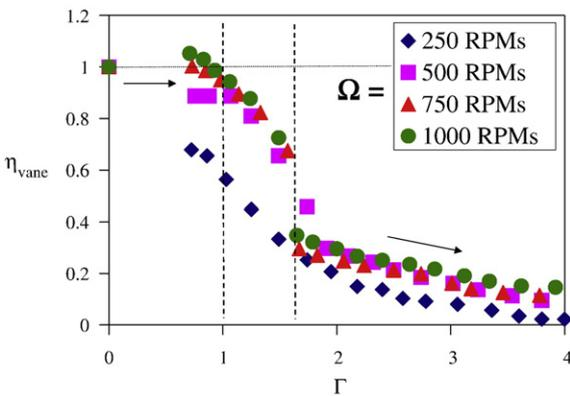
**Fig. 8.** Dimensionless vane power,  $\eta_{\text{vane}}$ , for increasing dimensionless vibration acceleration,  $\Gamma$ . The granular bed state behavior shown by  $\eta_{\text{vane}}$  for  $\Gamma$  increase is similar to  $\Omega$  increase in Fig. 3.
