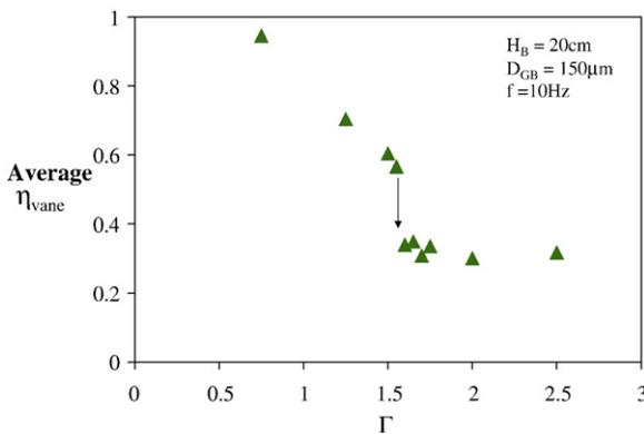
**Fig. 4.** The dimensionless vane power,  $\eta_{\text{vane}}$ , in Fig. 3 is a much weaker function of  $\Omega$  above 500 rpm. The average  $\eta_{\text{vane}}$ , are plotted vs. the dimensionless vibration acceleration,  $\Gamma$ , above. The quasi-static and vibro-fluidized bed states demonstrate the same behaviors for average  $\eta_{\text{vane}}$  vs.  $\Gamma$  that were previously shown for  $\eta_{\text{vane}}$  vs.  $\Omega$ .
