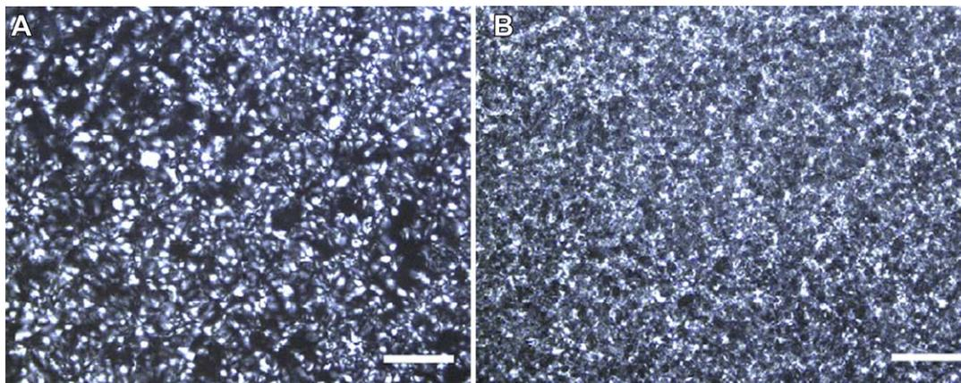
FIG. 7. Crystal morphology of neat HDPE (A) and HDPE/UHMWPE (B) composites after 50 min at 129°C. The white bar is 50  $\mu\text{m}$ . (Reproduced from Ref. 4, with permission from Elsevier). [Color figure can be viewed in the online issue, which is available at [wileyonlinelibrary.com](http://wileyonlinelibrary.com).]
